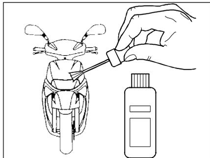
Minor paint damage should be immediately repaired.
